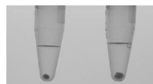
Fig. 1: recommended pellet sizes Left: maximum pellet size for turbidity from microbes Right: maximum pellet size for other turbid samples
